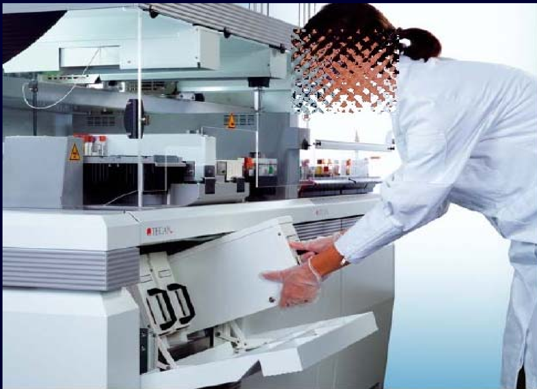
All blood samples are initially identified by the Tecan FE500 robot that sorts samples for diagnostic routine and samples dedicated to the BioBIM
